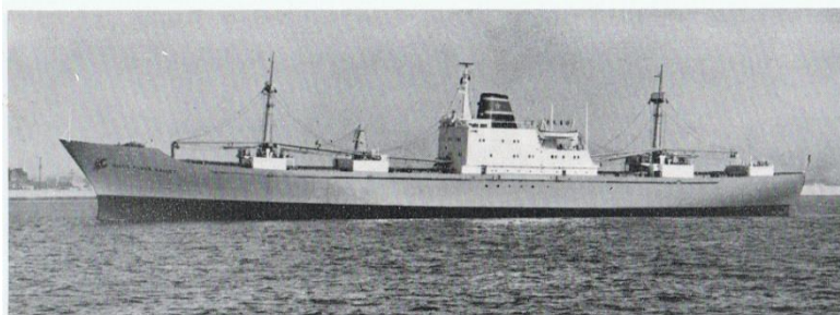
MS HOOD RIVER VALLEY Refer built by Blohm & Voss, Hamburg for Rederi AB Nord- stjernen (Johnson-Line), Stockholm. Delivered, February 8, 1965. Length o.a. . . . 449'8" (137.05 m) length b. p.p. 406'10" (124.00 m) beam, moulded . . . 57'1" (17.40 m) depth to upper d. 37'3" (11.35 m) draft (summer) 25'5" (7.74 m) deadweight, tons . . . . . 5,955 reefer capacity, cbf. baie 295,800 speed, knots . . . . . 20.5 MAN-diesel, K8Z70/120 D Power, EHP. . . . . 3,600 at r.p.m. . . . . 135 bore/stroke, mm . . . . . 700/1,200
